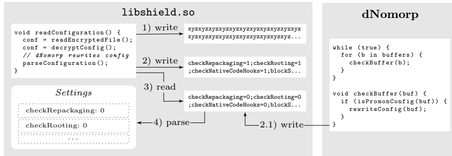
Fig. 4: Visualization of rewriting Promon Shield's configuration at runtime.
